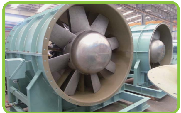
희석 fan(Dilution air fan)
